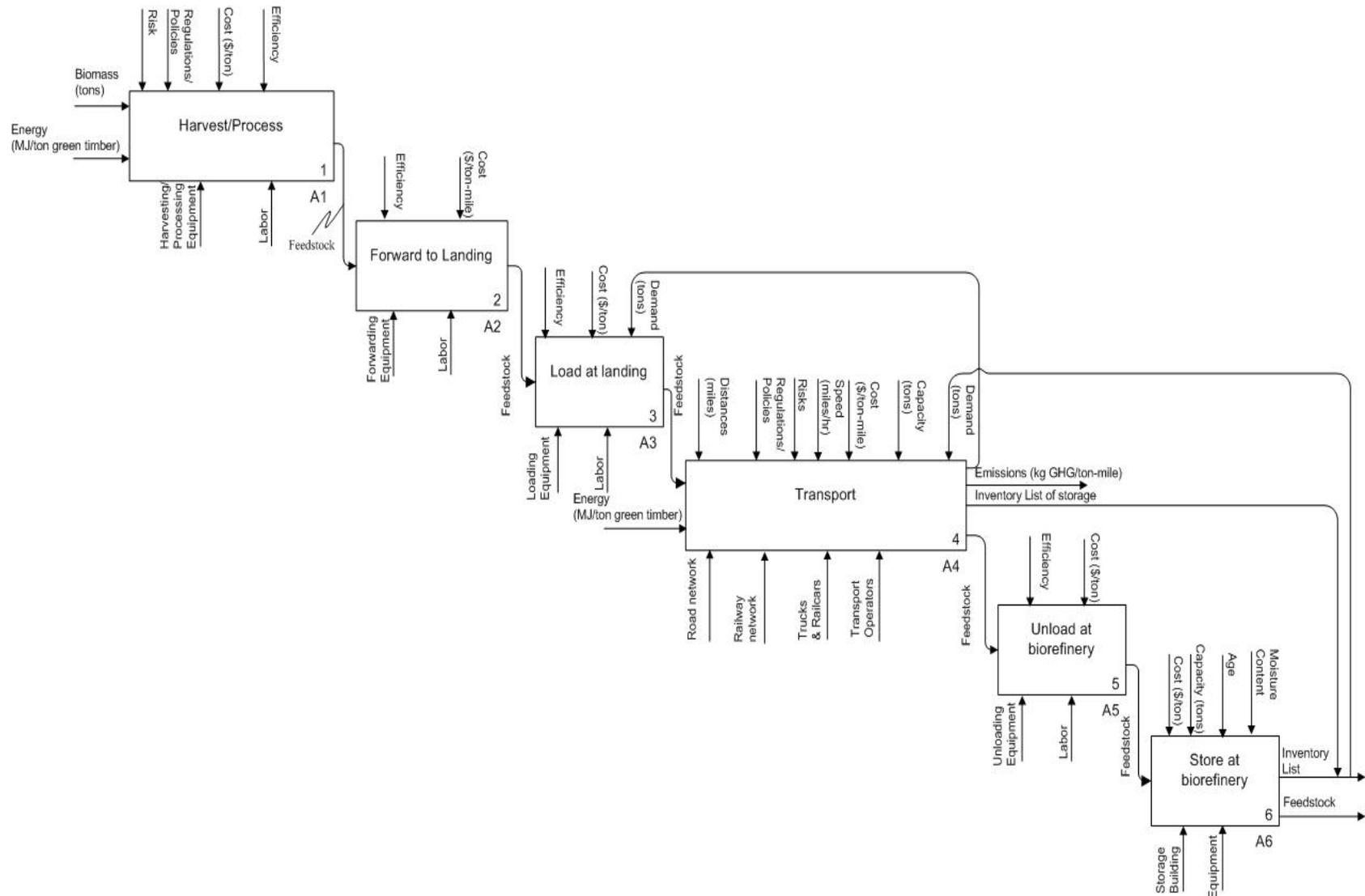
Figure 13 Complete Biomass Feedstock Supply Chain Model
