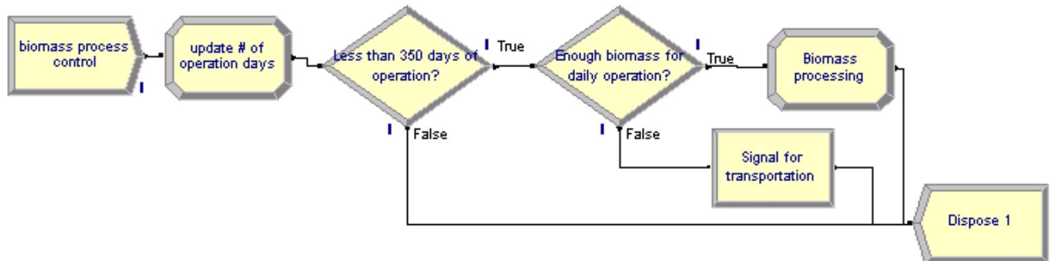
Figure 19 Sub-model Design for Biomass Processing
