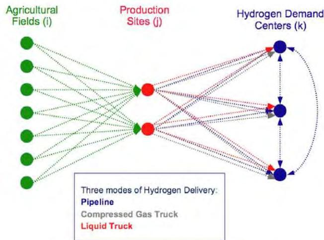
Fig. 2. Network representation of biohydrogen pathway.
