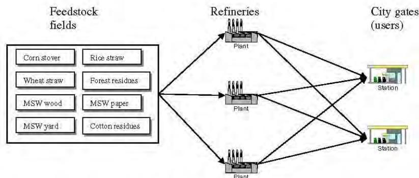
Fig. 1. A snap shot of a bioethanol supply chain.
