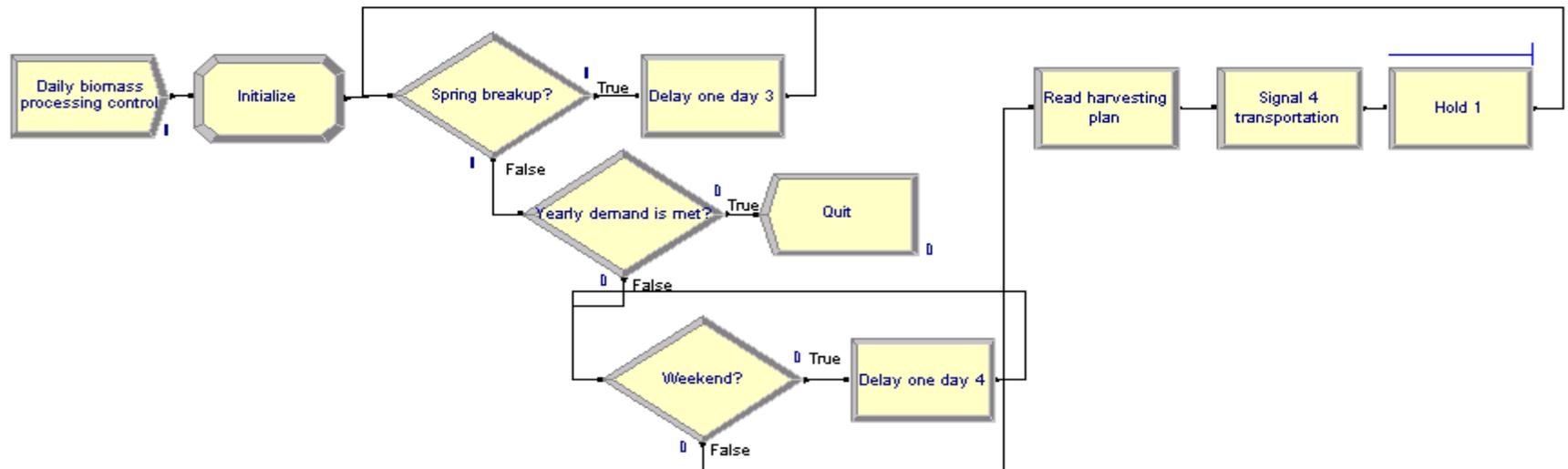
Figure 16 Sub-model Design for Reading Model Inputs
