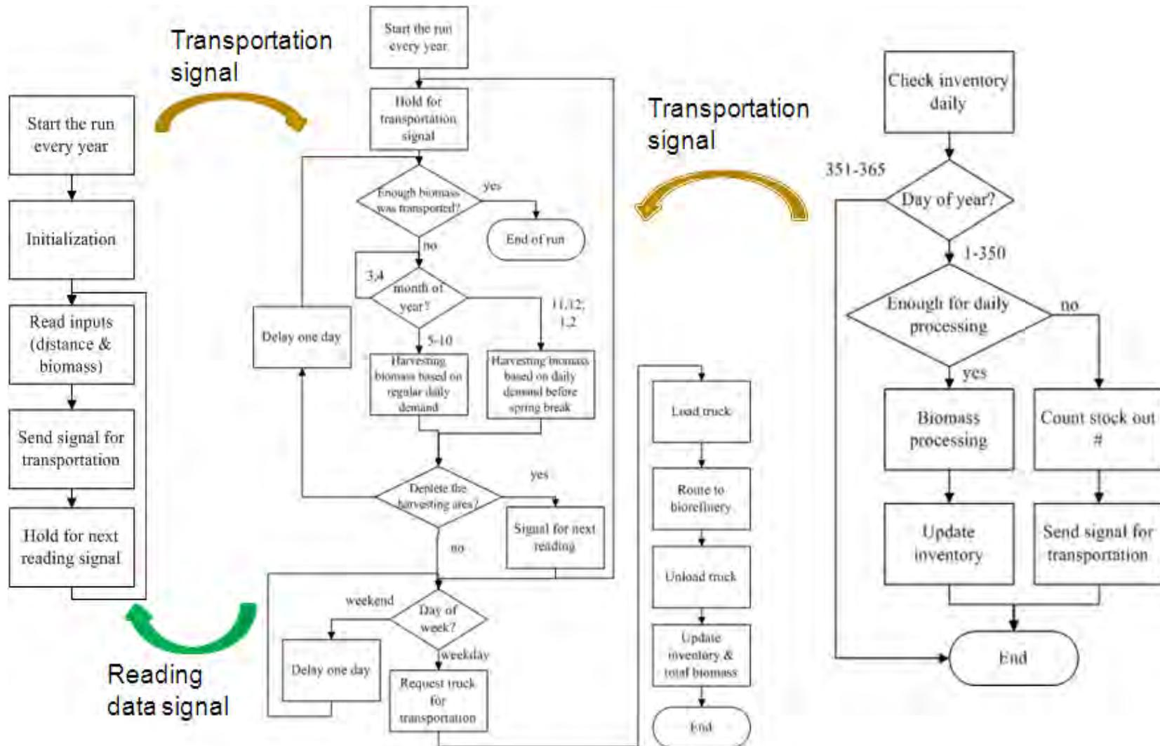
Figure 15 Logic for Biomass Supply Chain Model
